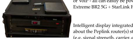
Intelligent display integrated in the case - displaying information about the Peplink router(s) status, cellular connectivity (e.g. signal strength, carrier, etc.) and much more with end-user
